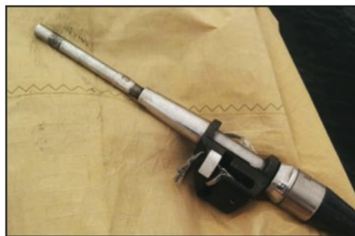
Top of the headstay where the stem ball fitting broke off.
